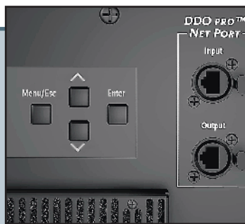
The DDO-Pro™ Net Port serves to network CTA 118 subwoofers via standard RJ 45 Ethernet plug-in connectors
