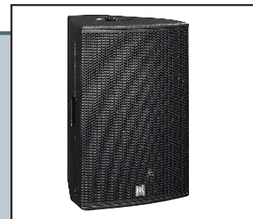
CT 115: 15"/1", 60° x 40° pivoting CD horn, 600 W RMS, 8 ohms, max SPL 134 dB
