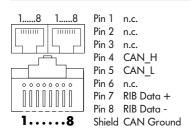
Fig. 11: Pin assignment for remote control (RJ45)
