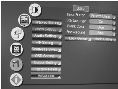
Figure 40: Advanced Utility Screen
